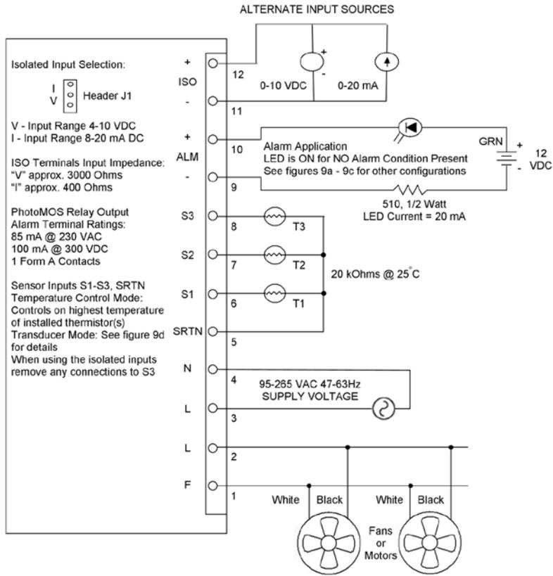
Figure 9: Wiring Diagram
