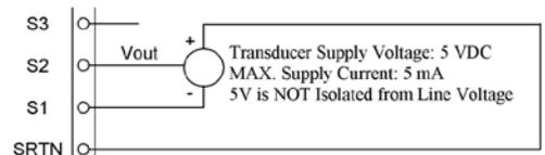
Figure 9d: Controlling with a Voltage Output Transducer
